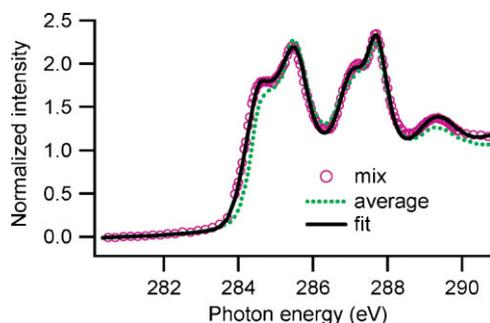
**Figure 5.** Experimental C K-edge spectrum of the binary layer (symbols), together with the arithmetic mean of the  $F_{16}CuPc$  and DIP spectra (dotted green line), and a fit to the data (solid black line). In the fit, the peaks of the fitted DIP spectrum, previously shifted rigidly by 0.2 eV, have been summed to the peaks of the fitted  $F_{16}CuPc$  spectrum. Then, only the intensities have been subject to minor adjustments.
