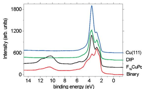
**Figure 4.** Valence-band photoelectron spectra taken with an excitation energy of 130 eV on the clean Cu(111) substrate, the single-component  $F_{16}CuPc$  and DIP layers, and on the binary layer.
