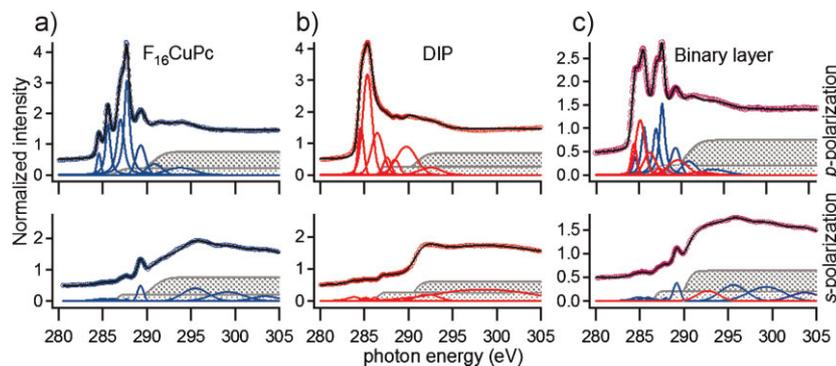
**Figure 3.** C K-edge NEXAFS spectra (symbols) of the single-component a)  $F_{16}CuPc$  and b) DIP layers, as well as c) that of the binary layer, under s- (bottom) and p-polarizations (top). The spectra have been fitted (solid line) with a number of peak and step functions represented under the corresponding spectra.
