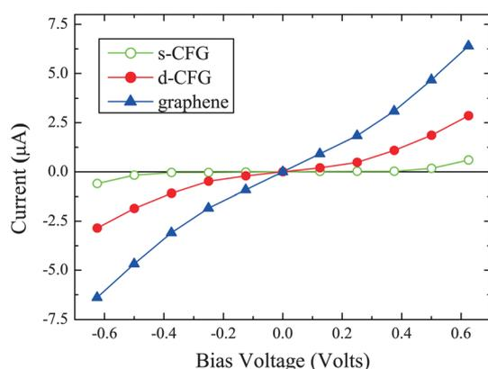
**Fig. 5** Current-voltage characteristics of s-CFG, d-CFG and the pristine graphene. The length of the scattering region is  $\sim 9 \text{ nm}$ .
