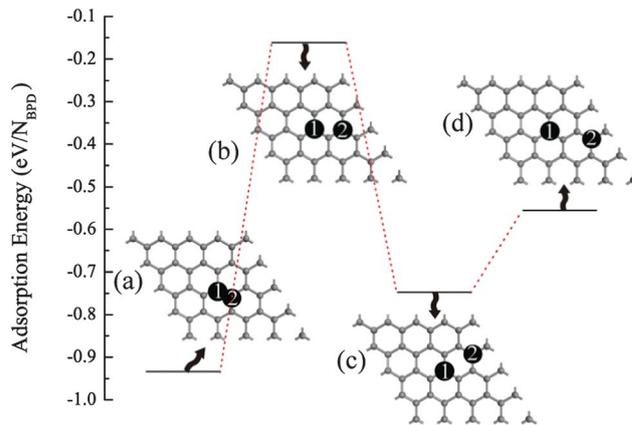
**Fig. 3** Adsorption energies for attaching the second TBP group on the opposite side of the graphene sheet in the  $4 \times 4$  supercell model. Four different configurations (a–d: ortho, meta, para, and neighboring ring) of d-CFG are considered, where black circles with numbers 1 and 2 represent the sites for the first and second TBP attachments, respectively.
