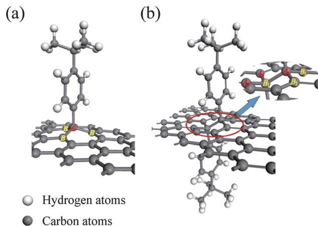
**Fig. 1** Optimized geometrical structures of (a) single-side functionalized graphene by TBP groups (s-CFG) and (b) double-side functionalized graphene by TBP groups (d-CFG). The graphene carbon atoms marked A and B belong to different sublattices.
