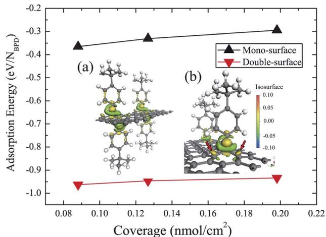
**Fig. 2** Calculated adsorption energy per TBP group for different surface coverage and charge density difference (in units of  $e \text{ \AA}^{-3}$ ) for (a) s-CFG and (b) d-CFG. The red arrows indicate the nearest-neighboring carbon atoms of the attachment site. The adsorption energy  $E_{\text{ad}}$  is defined as  $E_{\text{ad}} = (E_{\text{graphene}+n\text{TBP}} - E_{\text{graphene}} - nE_{\text{TBP}})/n$ , where  $n$  is the number of TBP groups.
