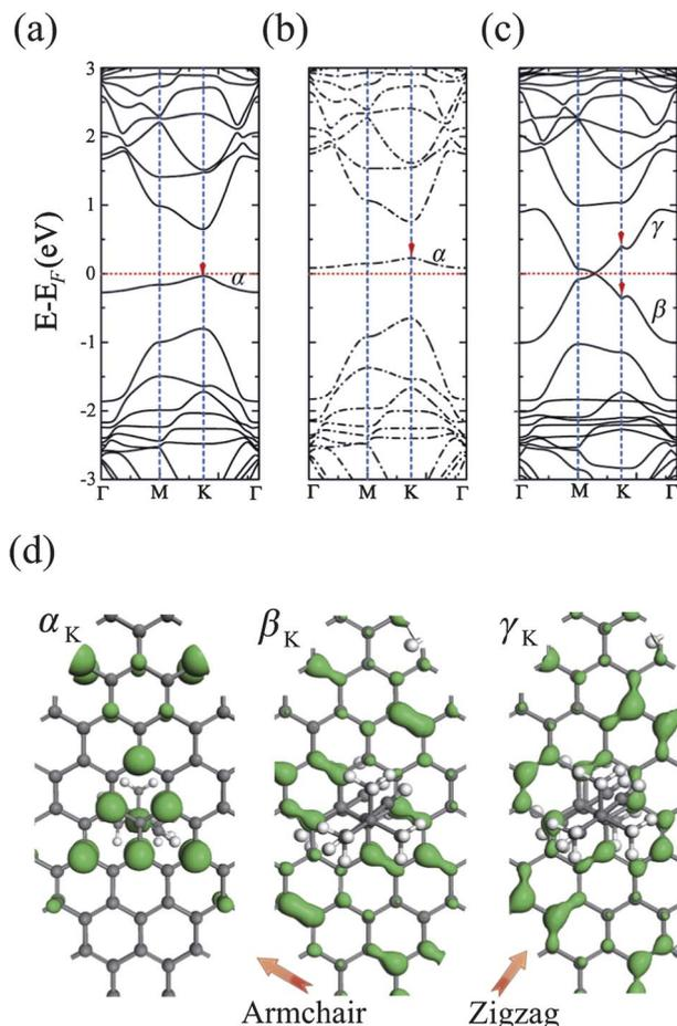
**Fig. 4** (a) Majority-spin and (b) minority-spin band structures of s-CFG with the coverage of  $0.20 \text{ nmol cm}^{-2}$ . (c) Band structure of d-CFG with the coverage of  $0.20 \text{ nmol cm}^{-2}$ . Fermi levels are set to zero. (d) Isosurfaces of charge density ( $0.03 \text{ e \AA}^{-3}$ ) of the  $\alpha$ ,  $\beta$  and  $\gamma$  bands at the K point.
