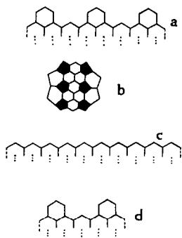
Fig. 3. Different types of tube ends mentioned at different times in the text. In (a), (c), and (d) the dashed bonds at the left and right are the same (the structure being bent into a circle to form a cylinder) and the tube structure continues onward (for a length  $L$ ) in the downward direction.
