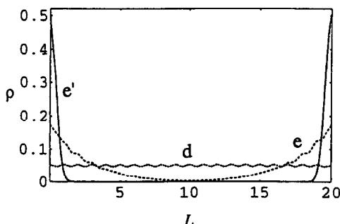
Fig. 4. Density vs. axial position for the frontier orbitals of  $(t_+, t_-) = (10, 0)$  tubes with length  $L = 20$ . The type (d) case is for a torus, the type (e) case is for a tube capped as in the inset of Fig. 1(b), with end-localized charge density, and the (e') case is for an open tube with completely end-localized charge density. These cases are correlated with the different behaviors of the band-gap shown in Fig. 1.
