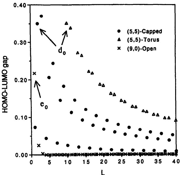
Fig. 1. Gap (in units of  $\beta$ ) vs. tube length  $L$  (in unit-cell lengths  $2.45 \text{ \AA}$  for  $(n,n)$  tubes and  $4.26 \text{ \AA}$  for  $(n,0)$  tubes), for different cases where the infinite tube has a zero-gap. There are two cases of  $(d_0)$  at  $(t_+, t_-) = (5, 5)$  and one case of  $(e_0)$  at  $(t_+, t_-) = (9, 0)$ ; the solid-dot  $(d_0)$  case involves a  $C_{5v}$  cap which is half of a buckminsterfullerene cage.
