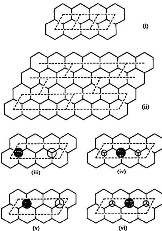
Fig. 5. In (i) the  $1 \times 3$  super-cell, and in (ii) their manner of interrelation. In (iii)–(vi) the four associated occupancy patterns for zero-energy orbitals, with open and shaded circles indicating opposite-signed amplitudes; in (iv) and (vi) the smaller circles correspond to half the amplitude of the larger ones.
