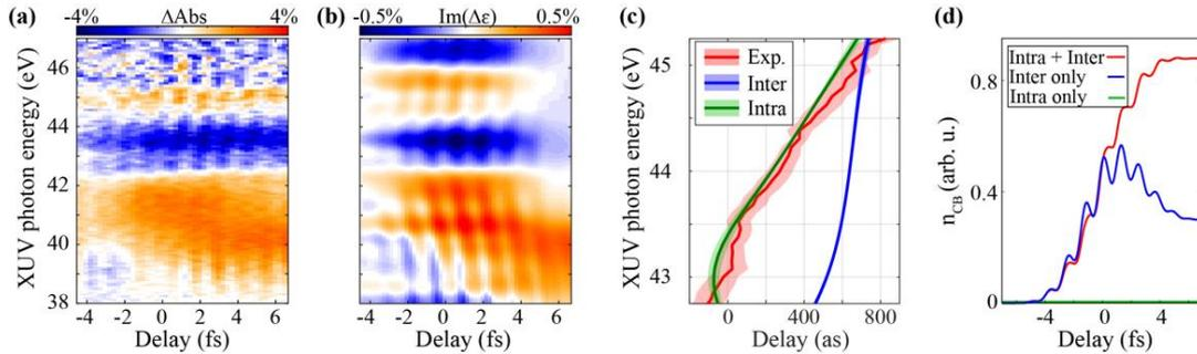
**Fig. 1** (a), (b) Measured and simulated transient absorption modulations induced by an intense *resonant* pulse. (c) Energy-dependent delay between the pump field intensity and transient absorption oscillations extracted from the measured signal and the simulations with only *intra*- or *inter*-band transitions included, respectively. (d) Simulated number of electrons excited from the VB into the CB for the different limits.
