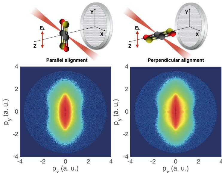
Fig.1: Sketch of the experimental arrangement with alignment of OCS molecules in the laboratory frame, parallel and perpendicular to the Y axis. The ionizing laser is linearly polarized along the Y axis and the detection is in the XY plane. The molecular-frame angle-resolved photoelectron spectra are projected onto a 2D detector in a velocity map imaging spectrometer.
