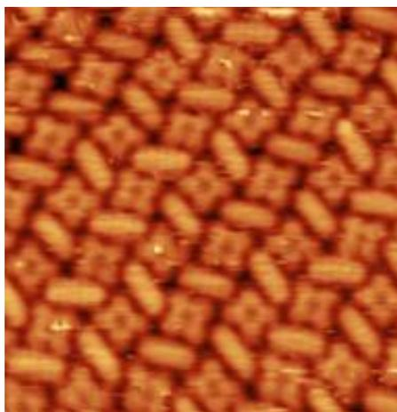
STM image of a self-assembled monolayer of PFP (acceptor) and CuPc (donor) on Ag(111) (13.2 nm<sup>2</sup>).
